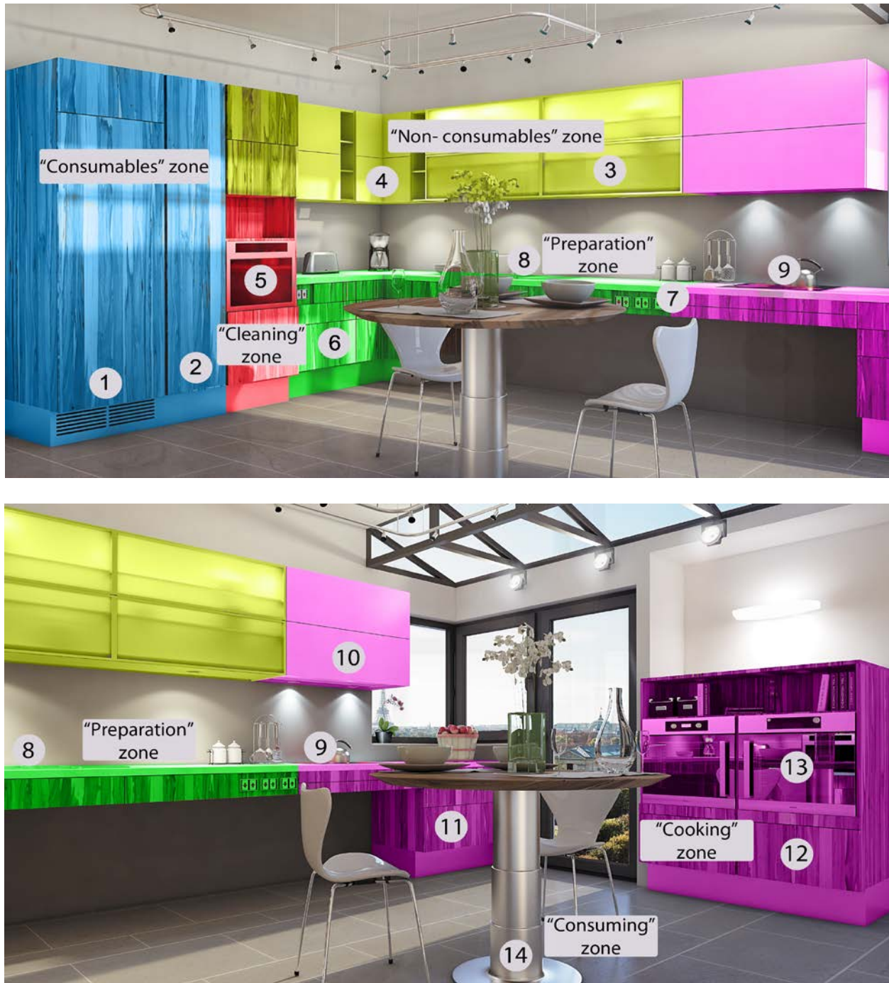
Fig. 4. Legend with design details of the presented “U- shaped” universal kitchen model
